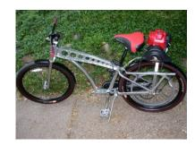
Figure 4 - A standard bicycle, retrofitted with a gaspowered motor.
