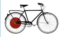
Figure 3 - A standard bicycle retrofitted with a Copenhagen Wheel E-bike system
