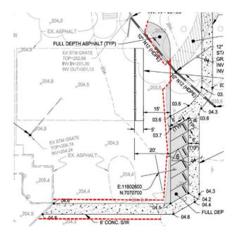
6. Contractor shall sawcut and remove asphalt as needed for installation of 10-inch drain piping.
