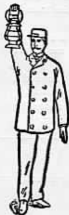
RELEASE AIR BRAKES—HELD AT ARM'S LENGTH ABOVE THE HEAD. SEE RULE 92 (f).
