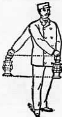
STOP—SWUNG ACROSS THE TRACK. SEE RULE 92 (a).
